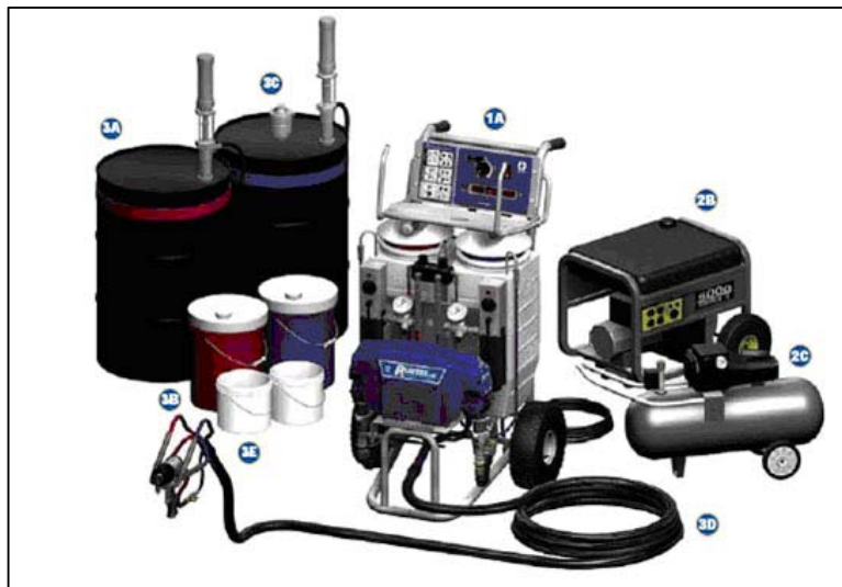
FIGURE 3 LOW PRESSURE EQUIPMENT
